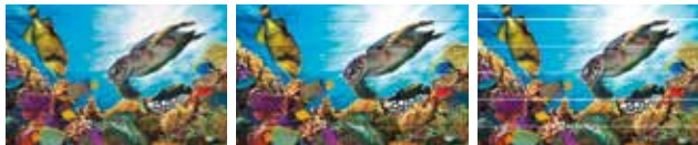
Incorrect bi-directional drop landing position Overlap / black streaks (Insufficient paper feeding) Gap / white streaks (Excessive paper feeding)
