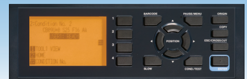
Intuitive 3.7" LCD Control Panel
